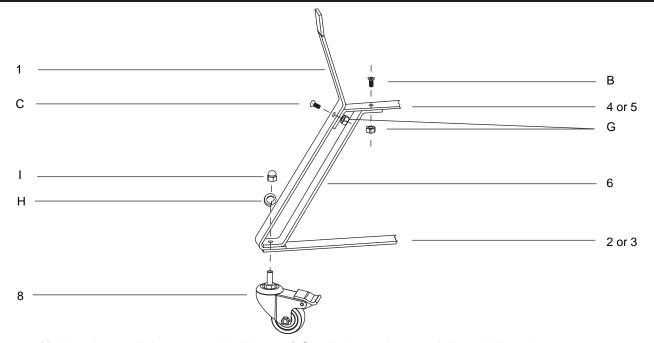
STEP 2 - (Joining the two halves assembled in step I) Stand the section 1 upright, and place the upper cross braces (4&5) close to section 1. Inserting truss head screw C through the hole of section1 and section 4&5 and install G nut and tighten securely.
