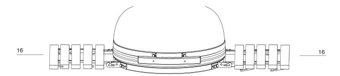
**STEP 16 -** Insert the 2x table hinge into each of the table brackets (17 & 18).
