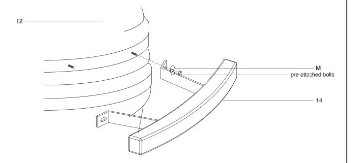
**STEP 10 -** Attach the lid handle (14) to the ceramic body (12), use the 2x pre-attached bolts with their corresponding washers, locking washers, and nuts per bracket.
