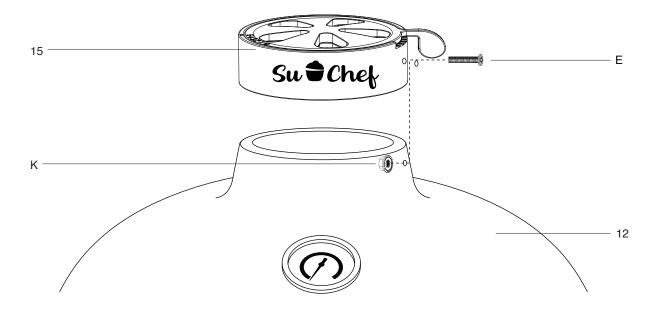
STEP 13 - To attach the top vent (15) to the Kamado Grill (12) place it on top and align both the bolt holes. Secure using 2x bolts (K) and nuts (E). Ensure that the top vent bolt is on the left hand side when assembling it.
